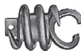
ROOT RIPPER Heavy spring screws into root mass, while front hook tears into stoppage PART # 75361228- 5/8" or 3/4" Cable
